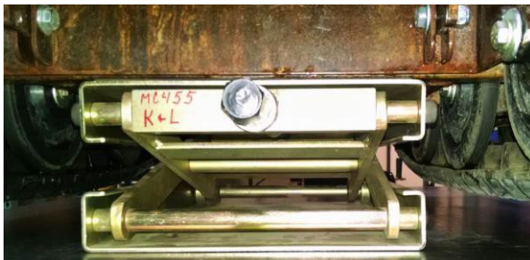
Elevate chair with suitable lift or blocks, here you see the K&L model MC455 fat jack.
